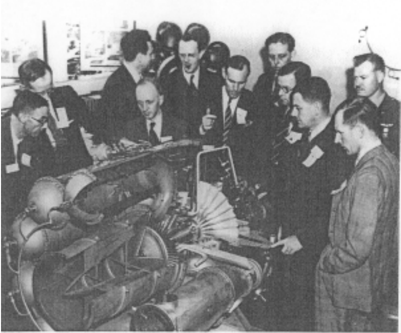
The British get a look at their modified “Whittle” engine, the A-1. GE engineers made a few modifications to the original design that increased efficiency.
